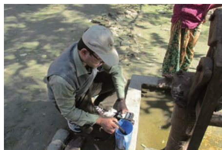
サンプル水の DO (溶存酸素) を湾岸部調査村で測定している Measurement of Dissolved oxygen of water from tube well in a coastal village of Bangladesh
