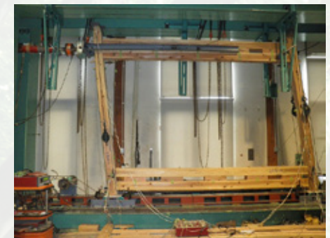
水平加力を受ける重ね透かし部材で構成された門型架構 Portal Frame Specimen composed of Spaced Built-Up Members Subjected to Lateral Loading
